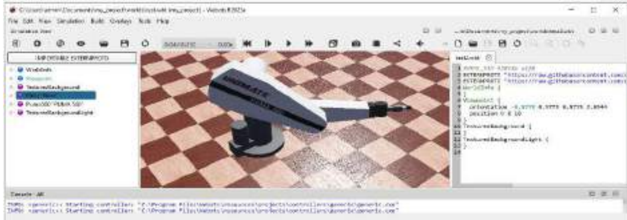
Figure 1. Webots simulation environment with industrial robot model and world editor.
